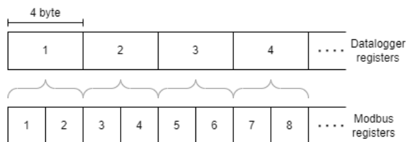
Figure 8.1: datalogger registers mapped to Modbus registers.
