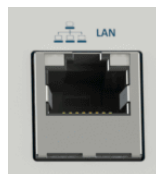
Figure 2.6: Ethernet RJ45 connector.
