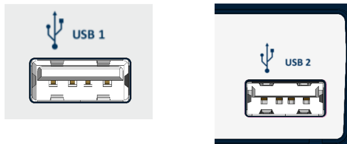
Figure3 .4 : front (USB 1) and side (USB 2) USB connectors.
