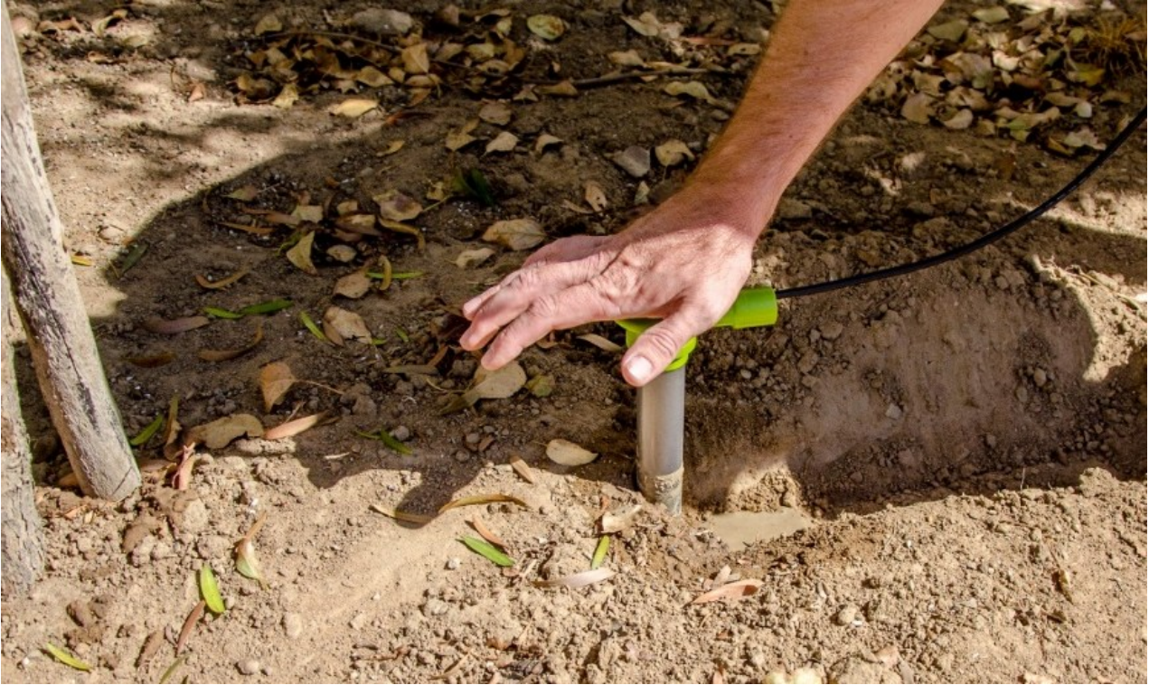
Figure 3. Installing the probe – Gently press down on the probe until it has reached the desired depth. Remove any access slurry.
