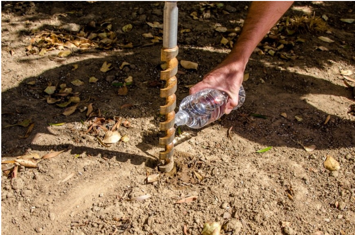
Figure 1. Drilling the access hole – A soil auger with 32 mm drill bit should be used. In dry compacted soils water can be added to ease the process.
